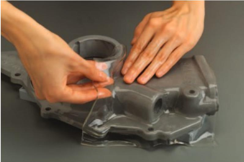
Figure 1. PhotoStress coating being contoured to the surface of a vehicle water pump casting
