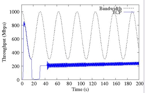
*After losses TCP is unable to quickly recover resources in large BDP networks: Alternatives to TCP have been proposed*
