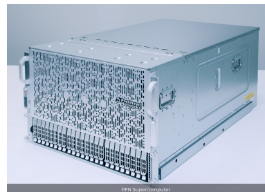
NM3 #1 Green500 : 1600cœurs – 2 Pflops – 55KW – 39 Gflops/watt
