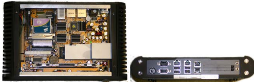
Fig. 1. Internal and connections views of the industrial autonomic network node.
