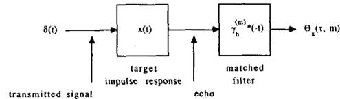
Fig. 2. Second receiver configuration using implicitly the transmitted signal  $h(t)$  of Fig. 1.
