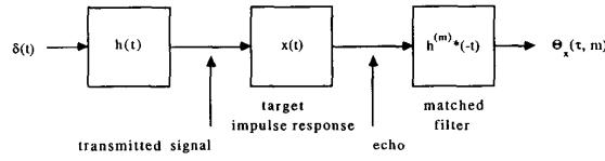
Fig. 1. First receiver configuration using explicitly a transmitted signal  $h(t)$ .
