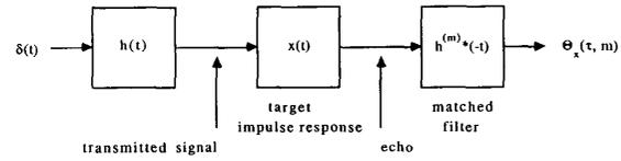
Fig. 1. First receiver configuration using explicitly a transmitted signal  $h(t)$ .
