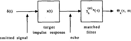
Fig. 2. Second receiver configuration using implicitly the transmitted signal  $h(t)$  of Fig. 1.
