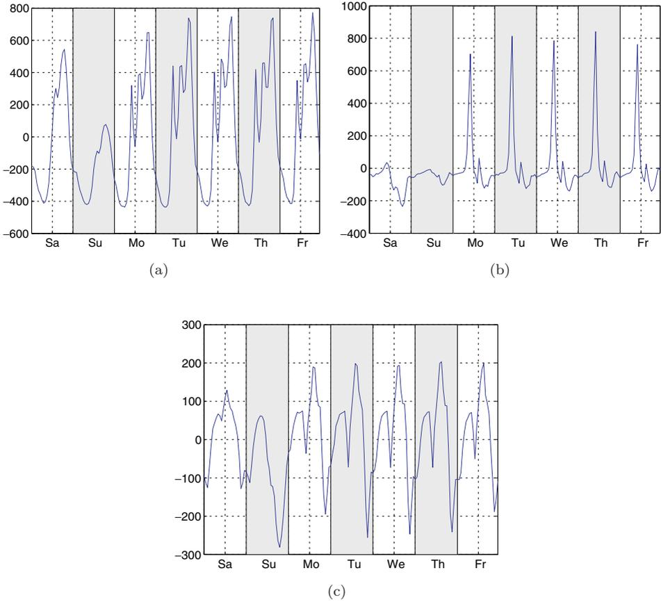
Fig. 11. **PCA analysis of  $T[m, n](t)$ .** The first 3 principal components of  $T$  are represented along time. One recognizes in the first one the cyclic part of the model,  $\langle L(t) \rangle_c$  (without its mean). The next components are mostly corrections on some of the peaks of this model: the second component changes mostly the mornings in the week-days, the third one brings corrections of opposite signs on noon and afternoon.
