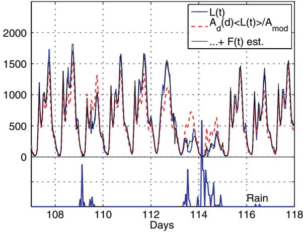
Fig. 8. **Hourly fluctuations of rental numbers: model and data.** The actual data (thin solid line), the model without the ARX(1) part (dashed line) and the full prediction with the ARX(1) part for  $\widehat{F}(t)$  are superimposed. On the bottom, the rain for these days is drawn (on arbitrary scale), showing that a major correction obtained by the ARX(1) is actually due to the rain.
