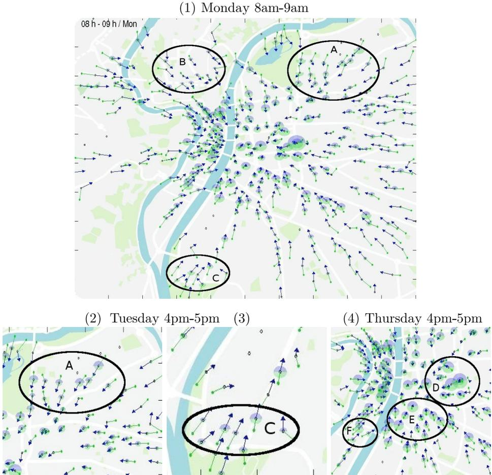
Fig. 4. (Color online) **Visualization of the traffic at all stations.** For a given hour, the amount of incoming and outgoing traffic is proportional to the area of the semi-circles at each station, incoming in light grey (green) on bottom; outgoing in dark grey (blue) on top. The arrow gives the average direction (as defined in Sec. 3.2) of these trips: incoming in light green; outgoing in dark blue arrow.
