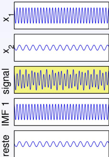
$$c\left(\frac{a_2}{a_1}, \frac{f_2}{f_1}, \varphi\right) = \frac{\|IMF_1(t) - x_1(t)\|_{\ell_2}}{\|x_2(t)\|_{\ell_2}}$$
