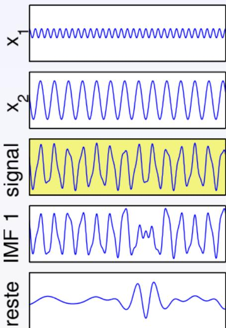
$$c\left(\frac{a_2}{a_1}, \frac{f_2}{f_1}, \varphi\right) = \frac{\|IMF_1(t) - x_1(t)\|_{\ell_2}}{\|x_2(t)\|_{\ell_2}}$$
