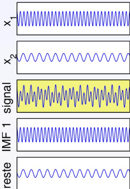
$$c\left(\frac{a_2}{a_1}, \frac{f_2}{f_1}, \varphi\right) = \frac{\|IMF_1(t) - x_1(t)\|_{\ell_2}}{\|x_2(t)\|_{\ell_2}}$$
