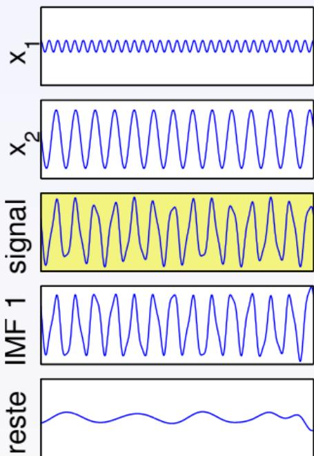
$$c\left(\frac{a_2}{a_1}, \frac{f_2}{f_1}, \varphi\right) = \frac{\|IMF_1(t) - x_1(t)\|_{\ell_2}}{\|x_2(t)\|_{\ell_2}}$$
