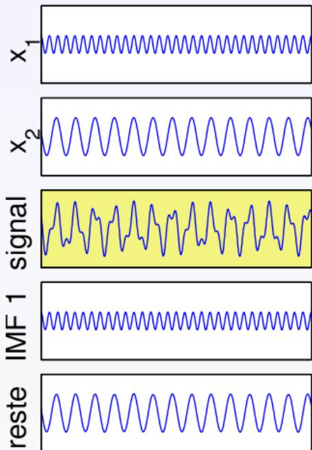
$$c\left(\frac{a_2}{a_1}, \frac{f_2}{f_1}, \varphi\right) = \frac{\|IMF_1(t) - x_1(t)\|_{\ell_2}}{\|x_2(t)\|_{\ell_2}}$$
