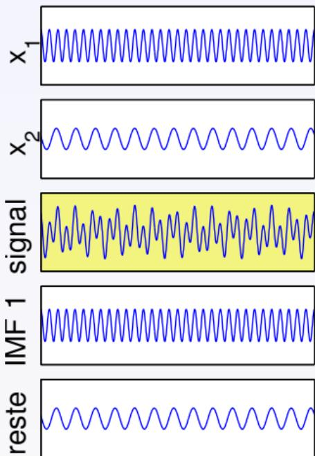
$$c\left(\frac{a_2}{a_1}, \frac{f_2}{f_1}, \varphi\right) = \frac{\|IMF_1(t) - x_1(t)\|_{\ell_2}}{\|x_2(t)\|_{\ell_2}}$$
