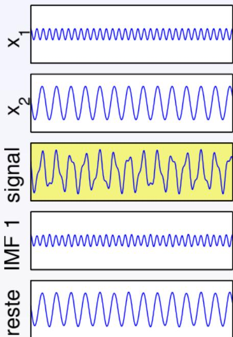
$$c\left(\frac{a_2}{a_1}, \frac{f_2}{f_1}, \varphi\right) = \frac{\|IMF_1(t) - x_1(t)\|_{\ell_2}}{\|x_2(t)\|_{\ell_2}}$$
