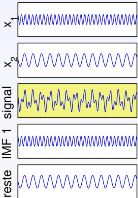
$$c\left(\frac{a_2}{a_1}, \frac{f_2}{f_1}, \varphi\right) = \frac{\|IMF_1(t) - x_1(t)\|_{\ell_2}}{\|x_2(t)\|_{\ell_2}}$$
