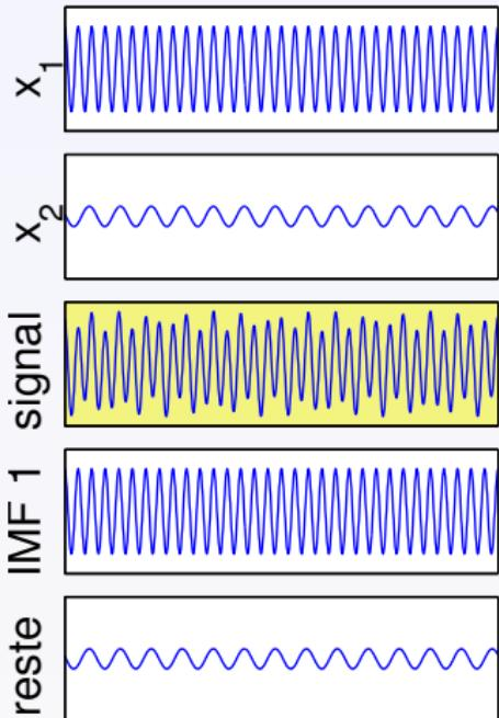
$$c\left(\frac{a_2}{a_1}, \frac{f_2}{f_1}, \varphi\right) = \frac{\|IMF_1(t) - x_1(t)\|_{\ell_2}}{\|x_2(t)\|_{\ell_2}}$$
