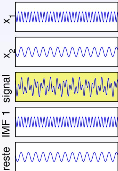
$$c\left(\frac{a_2}{a_1}, \frac{f_2}{f_1}, \varphi\right) = \frac{\|IMF_1(t) - x_1(t)\|_{\ell_2}}{\|x_2(t)\|_{\ell_2}}$$
