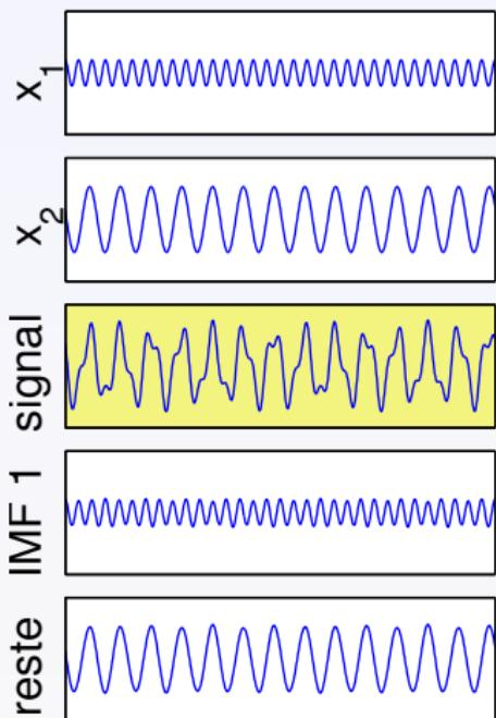
$$c\left(\frac{a_2}{a_1}, \frac{f_2}{f_1}, \varphi\right) = \frac{\|IMF_1(t) - x_1(t)\|_{\ell_2}}{\|x_2(t)\|_{\ell_2}}$$
