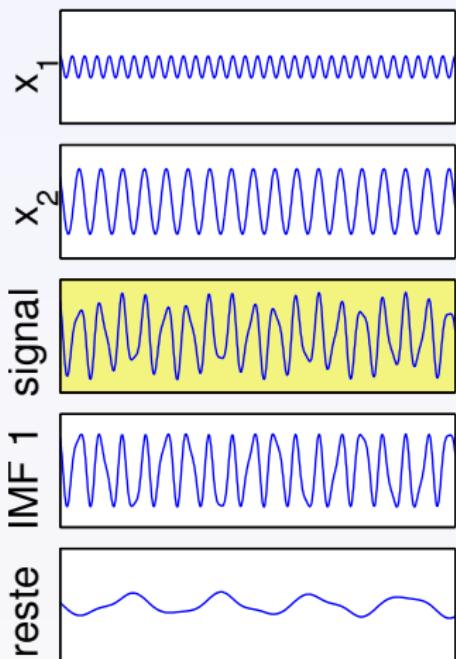
$$c \left( \frac{a_2}{a_1}, \frac{f_2}{f_1}, \varphi \right) = \frac{\|IMF_1(t) - x_1(t)\|_{\ell_2}}{\|x_2(t)\|_{\ell_2}}$$
