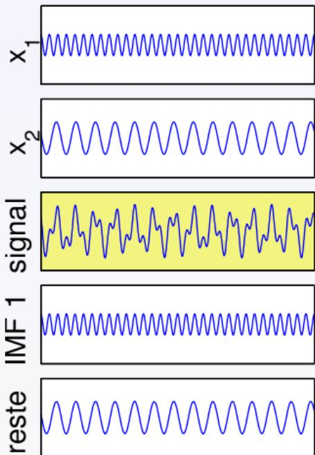
$$c\left(\frac{a_2}{a_1}, \frac{f_2}{f_1}, \varphi\right) = \frac{\|IMF_1(t) - x_1(t)\|_{\ell_2}}{\|x_2(t)\|_{\ell_2}}$$
