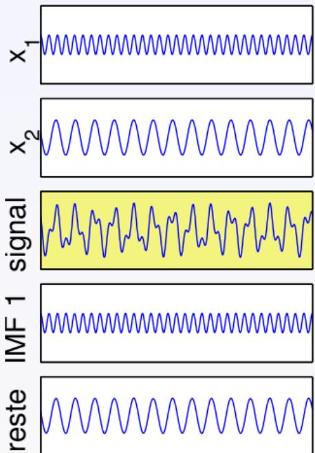
$$c\left(\frac{a_2}{a_1}, \frac{f_2}{f_1}, \varphi\right) = \frac{\|IMF_1(t) - x_1(t)\|_{\ell_2}}{\|x_2(t)\|_{\ell_2}}$$
