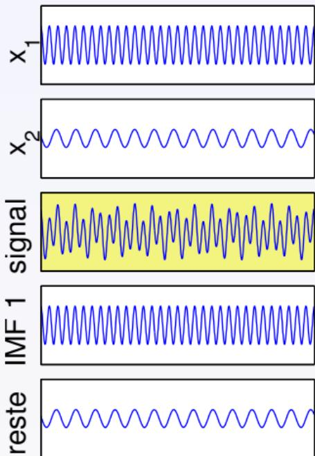
$$c\left(\frac{a_2}{a_1}, \frac{f_2}{f_1}, \varphi\right) = \frac{\|IMF_1(t) - x_1(t)\|_{\ell_2}}{\|x_2(t)\|_{\ell_2}}$$
