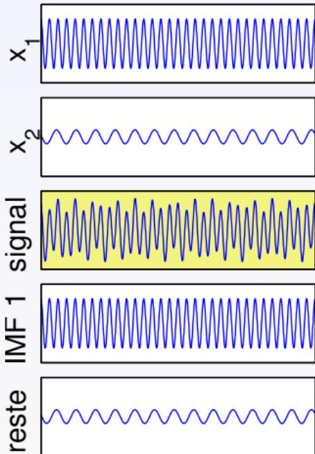
$$c\left(\frac{a_2}{a_1}, \frac{f_2}{f_1}, \varphi\right) = \frac{\|IMF_1(t) - x_1(t)\|_{\ell_2}}{\|x_2(t)\|_{\ell_2}}$$
