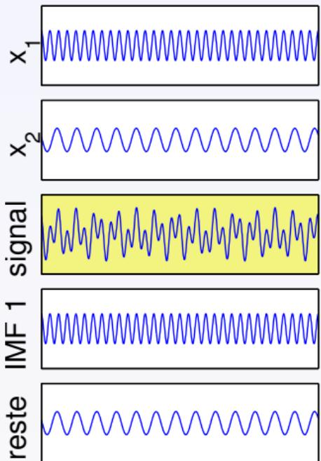
$$c\left(\frac{a_2}{a_1}, \frac{f_2}{f_1}, \varphi\right) = \frac{\|IMF_1(t) - x_1(t)\|_{\ell_2}}{\|x_2(t)\|_{\ell_2}}$$
