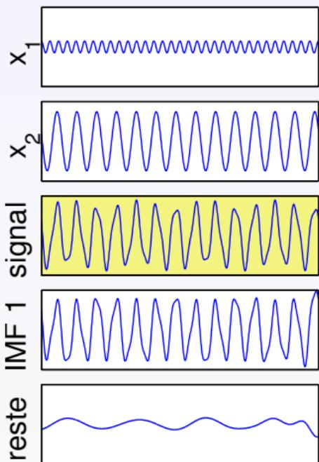
$$c\left(\frac{a_2}{a_1}, \frac{f_2}{f_1}, \varphi\right) = \frac{\|IMF_1(t) - x_1(t)\|_{\ell_2}}{\|x_2(t)\|_{\ell_2}}$$
