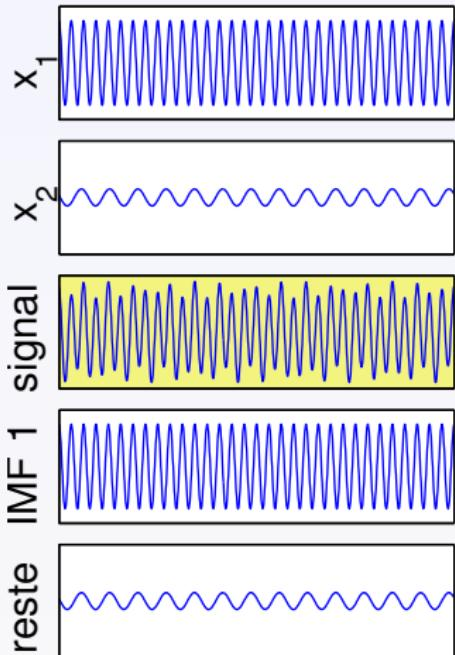
$$c\left(\frac{a_2}{a_1}, \frac{f_2}{f_1}, \varphi\right) = \frac{\|IMF_1(t) - x_1(t)\|_{\ell_2}}{\|x_2(t)\|_{\ell_2}}$$
