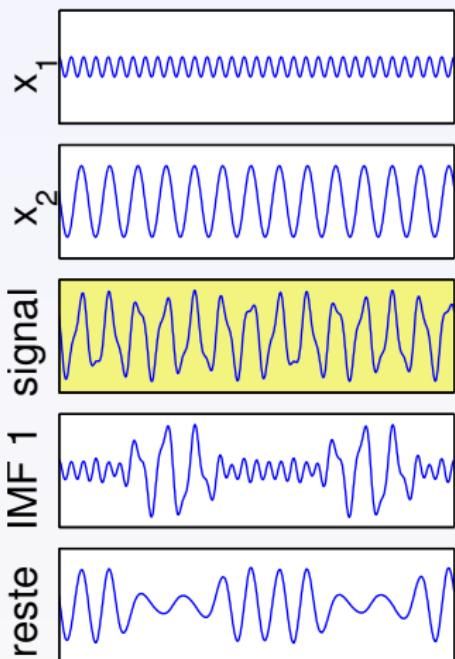
$$c\left(\frac{a_2}{a_1}, \frac{f_2}{f_1}, \varphi\right) = \frac{\|IMF_1(t) - x_1(t)\|_{\ell_2}}{\|x_2(t)\|_{\ell_2}}$$
