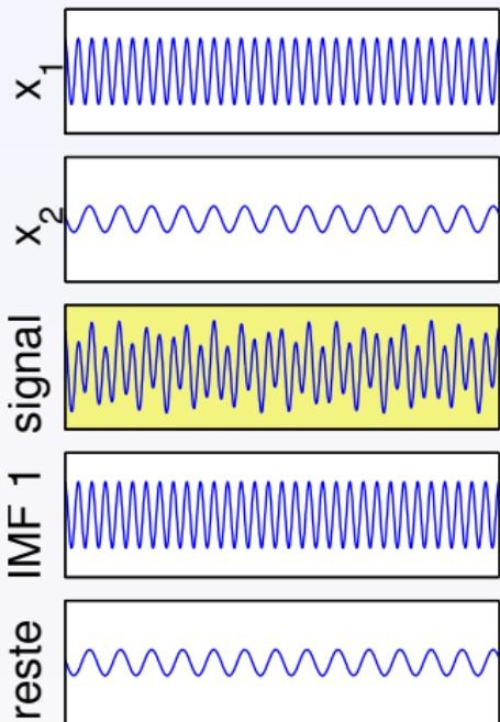
$$c\left(\frac{a_2}{a_1}, \frac{f_2}{f_1}, \varphi\right) = \frac{\|IMF_1(t) - x_1(t)\|_{\ell_2}}{\|x_2(t)\|_{\ell_2}}$$
