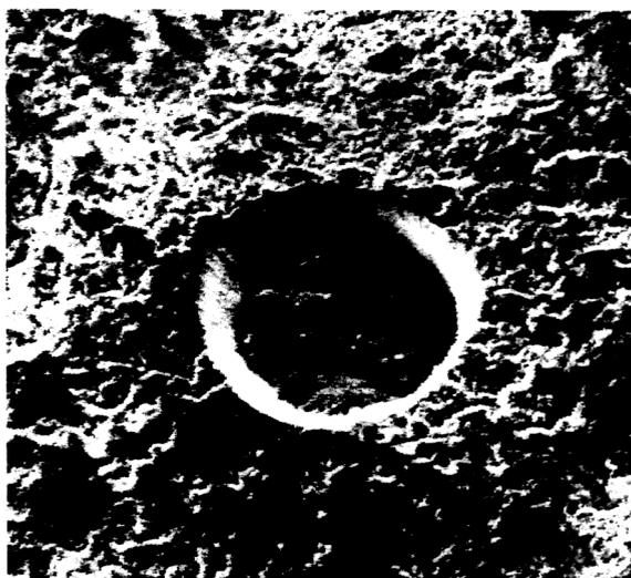
**Figure 1.** SEM photograph showing laser impact crater on NIST SRM 612 glass reference material. The crater shown had a diameter of 100 μm.
