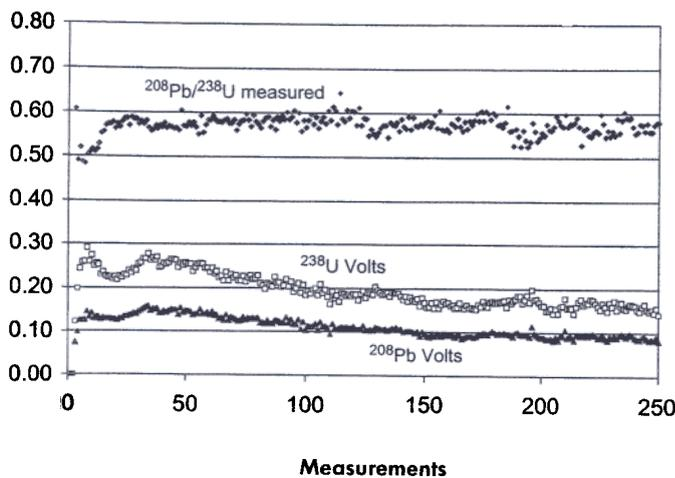
**Figure 4. Plasma 54 ICP-MS measurements on NIST SRM 610 for a 100  $\mu\text{m}$  crater at 10 Hz. Each symbol represents 2 seconds. The total acquisition time was 8 minutes.**
