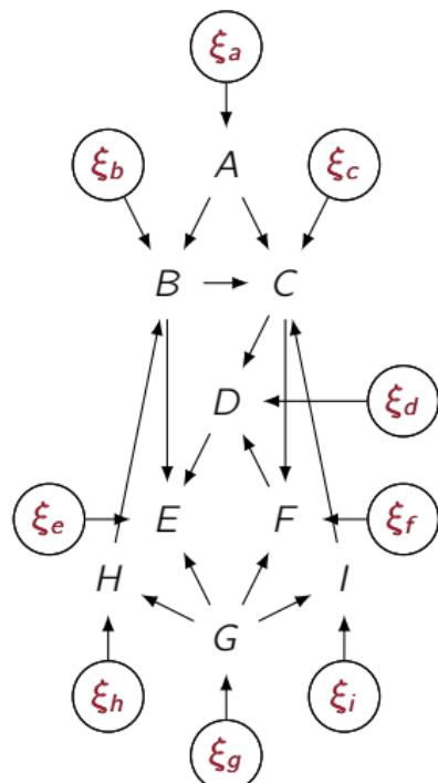
$$M : \left\{ \begin{array}{l} A := f_a(\xi_a) \\ B := f_b(A, H, \xi_b) \\ C := f_c(A, B, I, \xi_c) \\ D := f_d(C, F, \xi_d) \\ E := f_e(B, G, \xi_e) \\ F := f_f(C, G, \xi_f) \\ G := f_g(\xi_g) \\ H := f_h(G, \xi_h) \\ I := f_i(G, \xi_i) \end{array} \right.$$
