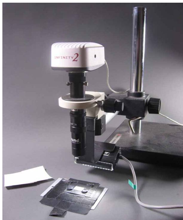
FIG. 1. System for raking-light close-up image acquisition.
