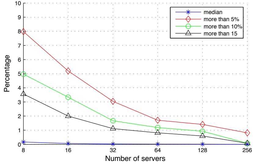
Fig. 5. Distribution of the percentage relative errors in the approximate solution for the loss probability in a Ph/Ph/c/N queue.
