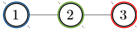
Figure 1: Conflict graph of a three-node network known as the Flow In the Middle (FIM) topology.
