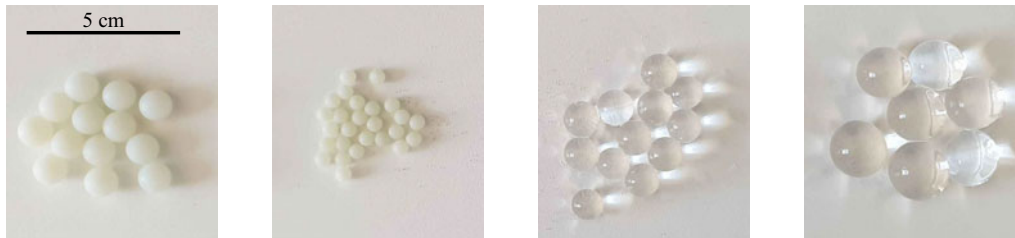
Figure 2. Particles used for the suspensions. From left to right: polyamide beads \sim 10 mm (PA10), polyamide beads \sim 5 mm (PA5), hydrogel beads \sim 10 mm (H10), hydrogel beads \sim 17 mm (H17). The scale is the same for all images. The characteristics of the particles are presented in table 1 .
