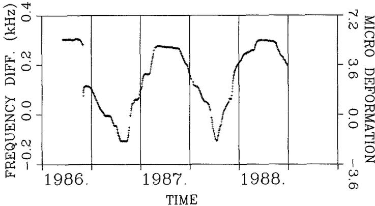
Fig. 7. Recorded frequency difference  $\Delta v$  for the same period of time as in the two previous Figures. The vertical scale on the left hand side is in kHz. On the basis of the calibration given in Fig. 4 this vertical scale is expressed as a deformation on the right hand side of the frame. The zero is arbitrary for both scales
