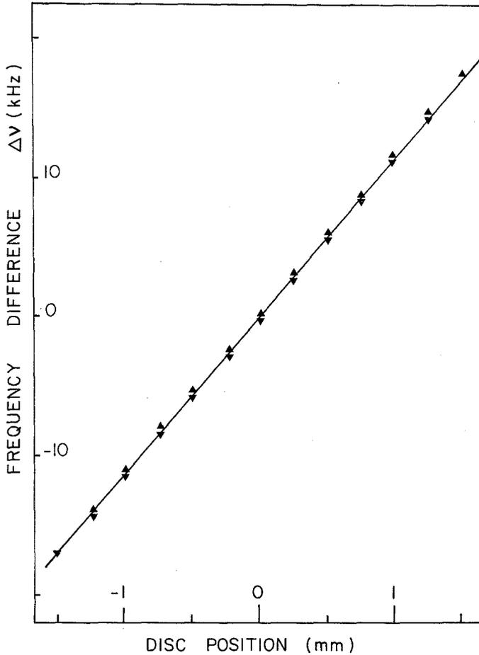
Fig. 4. Calibration curve showing the measured difference  $\Delta v$  between the resonance frequencies of the two LC circuits of the detector described by Fig. 2. This quantity is plotted vs. position of the metallic disc (3) away from the center between both coils. The small hysteresis is caused by some back lash in the micrometer device (5). The above numbers in brackets refer to Fig. 1
