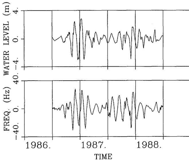
Fig. 8. Filtered water level (top) and deformation (bottom) curves obtained by removing all periods larger than 50 days in the data sets presented in Figs. 5 and 7. The time interval before July 1<sup>st</sup> 1986 which contains an artificial signal caused by a last calibration of the extensometer was left out of this Fourier analysis
