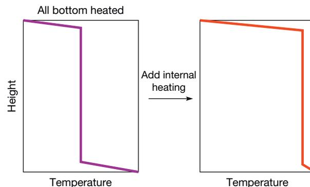
**Figure 8** Sketch of temperature profiles, as in Figure 6, for an isoviscous plane layer, with and without internal heating. With no internal heating, the interior mean temperature is the average of the top and bottom temperatures; the effect of adding internal heating is to increase the interior mean temperature and thus change the relative size and temperature drop across the top and bottom thermal boundary layers.
