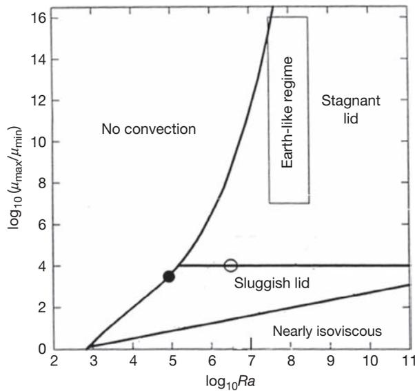
**Figure 12** Diagram showing the different convective regimes in 'Ra versus viscosity ratio' space for convection in fluid with temperature-dependent viscosity;  $\mu_{\max}$  and  $\mu_{\min}$  are the maximum and minimum allowable viscosities of the fluid, respectively. See text for discussion. Adapted from Solomatov V (1995) Scaling of temperature dependent and stress dependent viscosity convection. *Physics of Fluids* 7: 266–274.
