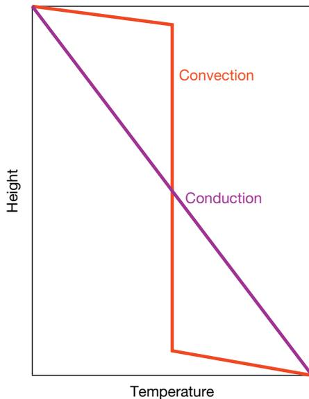
**Figure 6** Sketch of temperature profiles (i.e., horizontally averaged temperature vs. depth) for a simple isoviscous basally heated plane layer. Convective mixing homogenizes the conductive mean temperature into a nearly isothermal state (if the fluid is incompressible) with thermal boundary layers connecting it to the cold surface and hot base.
