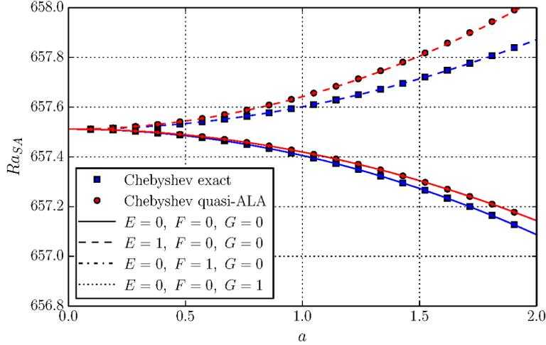
FIGURE 19. Linear stability critical threshold for the Rayleigh number for a generic EoS (8.27) as a function of the temperature gradient  $a$  of the base linear solution, for a negligible  $\mathcal{D} = 10^{-8}$ . The labels are identical to those defined in Fig. 18.
