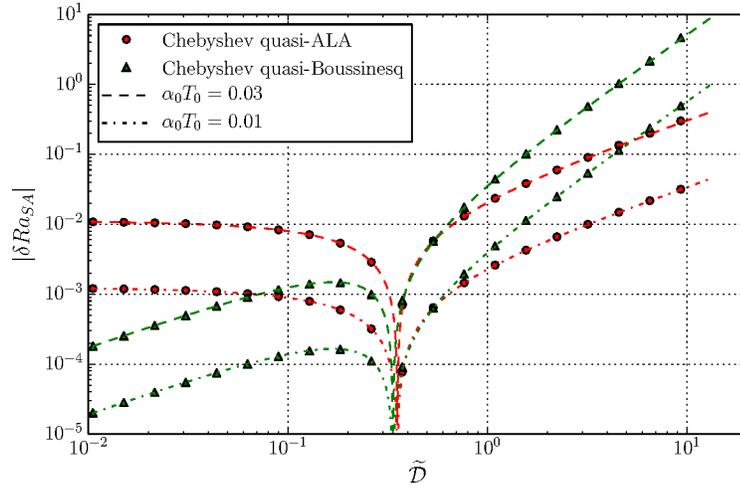
FIGURE 16. Similar to Fig. 13 but in logarithmic coordinates and for the absolute difference of the critical Rayleigh numbers between the approximations and exact model, for two values of  $\alpha_0 T_0 = \hat{\alpha}$  (0.03 and 0.01) and  $\gamma_0 = 1.03$ .
