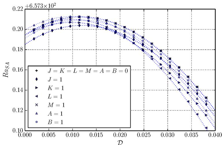
FIGURE 25. Same as Fig. 24 with a close-up around small values of  $\mathcal{D}$ , between 0 and 0.04. It is clearly visible that all parameters have an impact on the critical Rayleigh number, except  $M$  (+ and  $\times$  symbols superimpose), as predicted by the approximate analysis.
