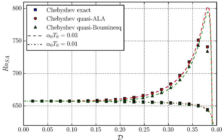
FIGURE 13. Linear stability critical threshold for the Rayleigh number for a Murnaghan EoS as a function of the dissipation number  $\mathcal{D}$ , for a fixed temperature gradient  $a = 0.4$  (corresponding to a temperature ratio  $r = 1.5$ ). The labels are defined on Fig. 12.
