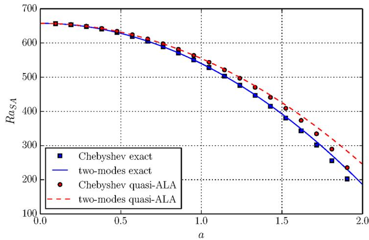
FIGURE 3. Linear stability critical threshold for the Rayleigh number for an ideal gas as a function of the temperature gradient  $a$  of the base linear solution, for a negligible  $\mathcal{D} = 10^{-8}$  and a ratio of heat capacities  $\gamma$  equal to  $5/3$ . Labels and linestyles correspond to that of Fig. 2.
