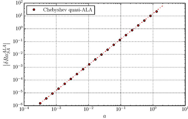
FIGURE 6. Absolute difference between the quasi-ALA critical Rayleigh number and the exact critical Rayleigh number, for an ideal gas as a function of  $a$ , for  $\mathcal{D} = 10^{-8}$  and three values of the ratio of heat capacities,  $\gamma = 5/3$ ,  $9/7$  and  $13/11$ . The results using these three values are undistinguishable as expected from the approximated solutions (8.12) and (8.13).
