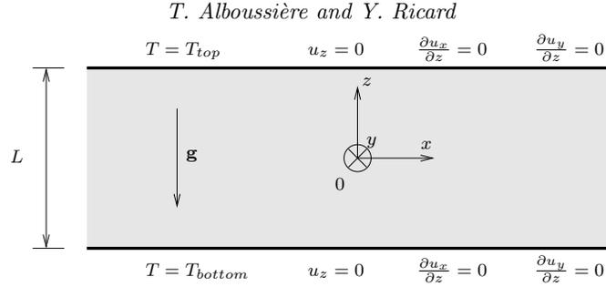
FIGURE 1. Rayleigh-Bénard configuration, with imposed temperatures and tangential stress-free boundary conditions
