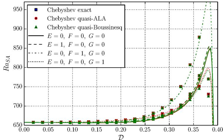
FIGURE 21. Linear stability critical threshold for the Rayleigh number for a generic EoS (8.27) as a function of the dissipation number  $\mathcal{D}$ , for a fixed temperature gradient  $a = 0.4$  (corresponding to a temperature ratio  $r = 1.5$ ). The labels are similar to those in Fig. 20.
