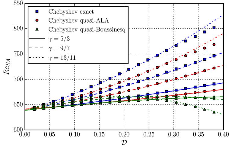
FIGURE 5. Linear stability critical threshold for the Rayleigh number for an ideal gas as a function of the dissipation number  $\mathcal{D}$ , for a fixed temperature gradient  $a = 0.4$  (corresponding to a temperature ratio  $r = 1.5$ ). The labels and linestyles correspond to those of Fig. 4.
