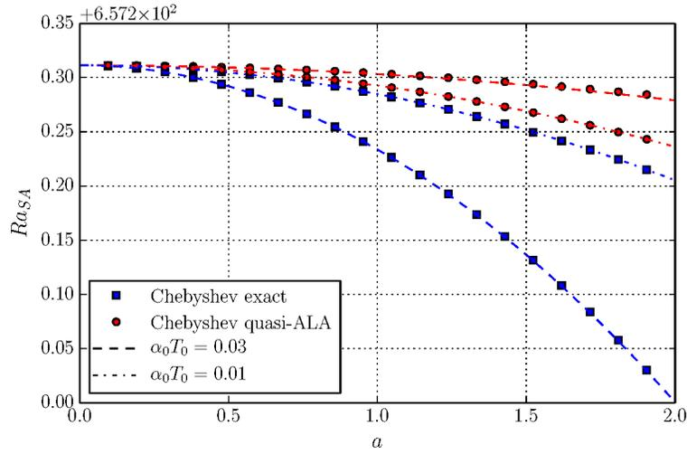
FIGURE 11. Linear stability critical threshold for the Rayleigh number for a Murnaghan EoS as a function of the temperature gradient  $a$  of the base linear solution, for a negligible  $\mathcal{D} = 10^{-8}$ . The labels are similar to those of Fig. 10.
