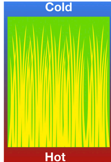
Fig. 3. The ambient phase (in green) is a porous deformable matrix in which the much less viscous fluid (in yellow), percolates. The mixture is submitted to a temperature gradient. (For interpretation of the references to colour in this figure legend, the reader is referred to the web version of this article.)
