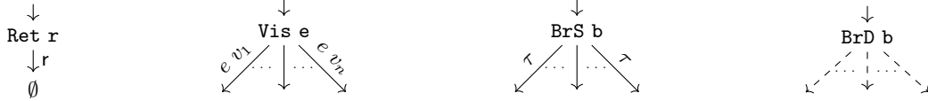
Figure 1 The four kinds of nodes in values of type ctree E B X . r value of type X , e external event taken from E , and b external or internal branching taken from B . The edge labels hint at the LTS the structure represents.
