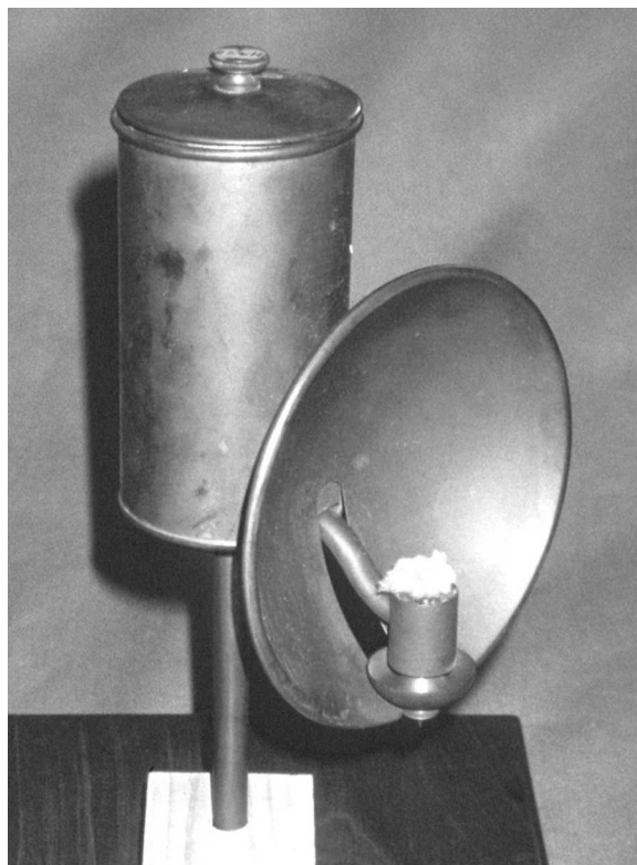
Locatelli's Lamp. Locatelli's lamp was used as a source for experiments on thermal radiation. The lamp burns alcohol in the wick placed at the focal point of the polished copper reflector. There is no chimney, and the cylindrical tank holds the alcohol. This lamp, from the Greenslade Collection, was sold by Max Kohl of Chemnitz for 14.50 marks at around 1900. It is shown in the Kohl catalogue as part of a complete set of apparatus that was mounted on an optical bench. (Photograph and notes by Thomas B. Greenslade, Jr., Kenyon College)
