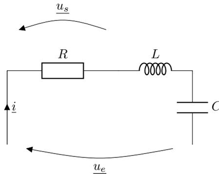
$$\underline{H} = \frac{\underline{u}_s}{\underline{u}_e} = \frac{jRC\omega}{1 + jRC\omega - LC\omega^2} \quad (24)$$
